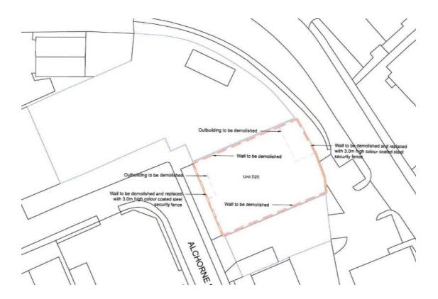
2.5 Existing brick walls in and around the site are to be demolished to enable the new boundary treatments to be installed and remain secure. The site does not fall within a conservation area and has no heritage designations and as such the demolition of existing walls does not require planning permission (it is Permitted Development). Consent is sought for the demolition of the two small buildings.
